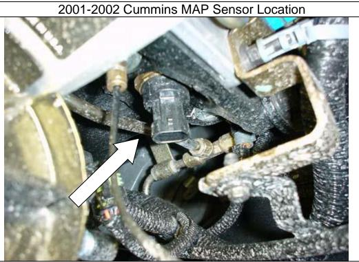
Note: The 2002 Cummins motor will have gray plug in same position.
